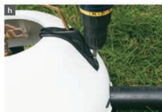
Screw wire clip holders into the holes provided.
