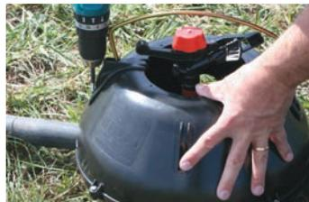
Screw wire clip holders into the holes provided.
