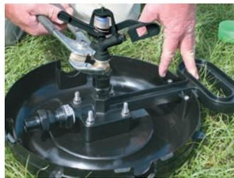
Screw the 20mm sprinkler into the socket.
