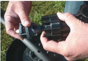
Tip the Pop-up TST until Mini Reg or Riser protrude, hold with finger and screw on Nelson R2000WF. Note all threads should be hand tight, do not use a tool for tightening.
