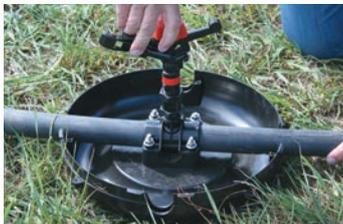
Screw sprinkler into Hansen Socket on riser.
